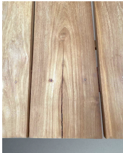
examples of cracking in teak wood
